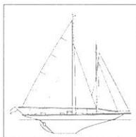
**Bermudan or Marconi yachts** have triangular mainsails fastened on two sides to the mast and boom. Even if it not entirely correct, they are also called Marconi rigged from the name given to the rig of Istria, the 15 m I.R. designed in 1912 by C.E. Nicholson and the first to use a mast in just one piece without the fore topgallant mast. The numerous stays used to support the mast made it resemble a radio antenna, which lead to the name.
