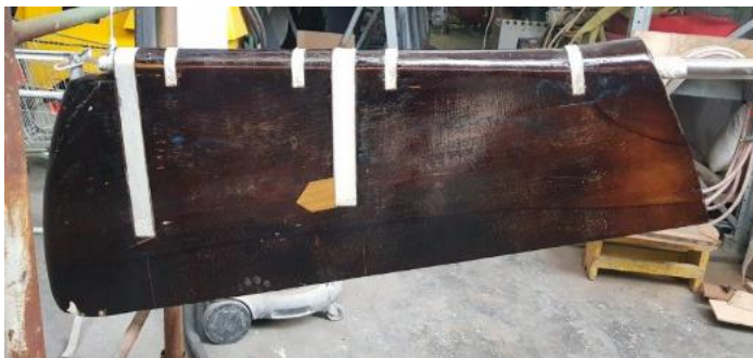
The rudder following its restoration. The light patch is an insert substituting rotten wood
