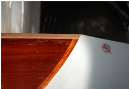
The transom as it appeared once the paint was stripped, and after restoration
