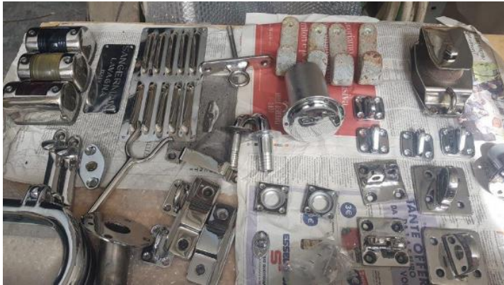
The original fittings cleaned and ready to be reinstalled
