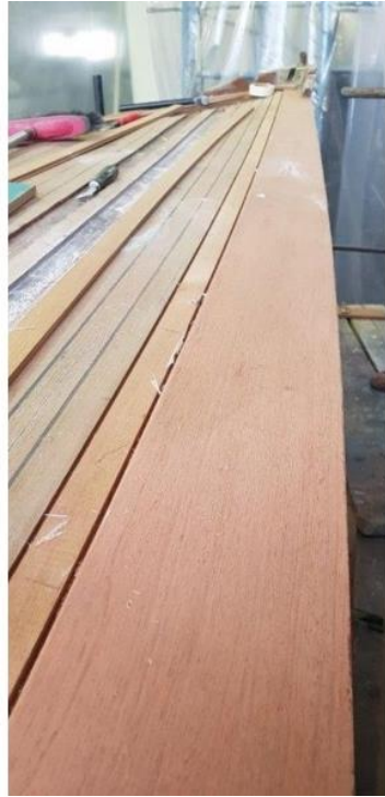
Left, the old gunwale has been removed and the underlying deck is plugged Right, the new gunwale, freshly installed
