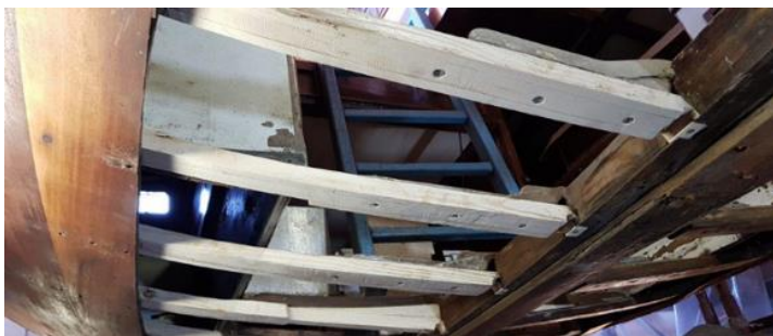
The frames, re-built or reinforced with ash wood
