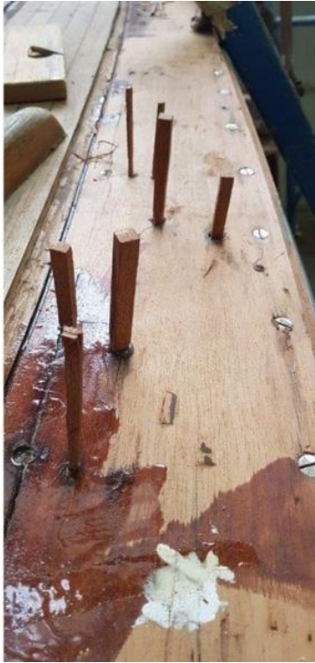
Left, the old gunwale has been removed and the underlying deck is plugged Right, the new gunwale, freshly installed
