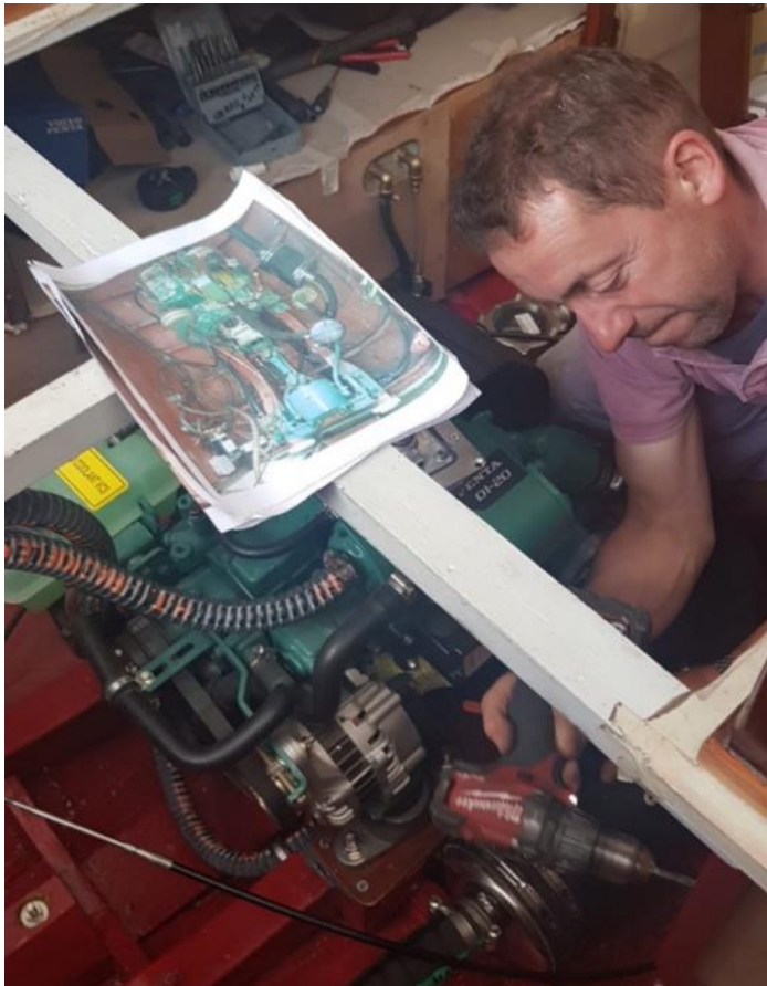
Installation of the new engine, a Volvo Penta 20 HP (14 KW)
