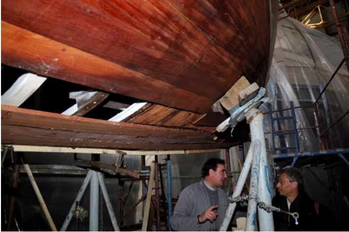
New mahogany planks substitute the ones rotten and removed. Marco Poirino explains the process
