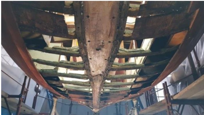
The hull minus the planks rotted courtesy of the fiberglass coat
