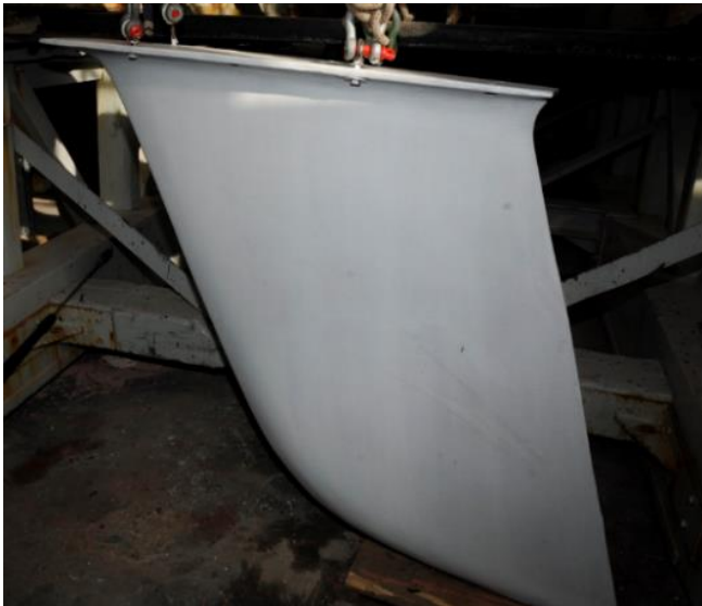
The keel cleaned, primed and ready to be re-installed
